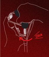
Always tighten until you hear a 'click'. Failure to do so may result in separation of the club head or product damage.
